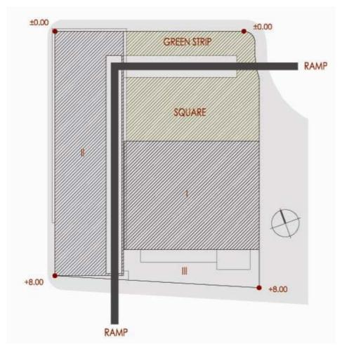
The west side of the site was judged as best for the approach of the vehicles to the building. Finally, at the north front of the lot there is a permanent parking area and the truck' access to the underground delivery maintaining area. the striped green space, which expands until the square, continuing the open green space of the lot 134-01.
